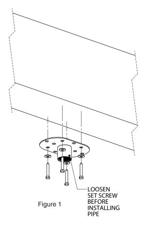
The MP-1.5NPS-CP provides a safe ceiling mounting plate for 1-1/2-11 NPS and NPT threaded pipes. The ceiling plate can be installed to most horizontal overhead structures, including ceiling trusses, beams, Unistrut and other structural components
