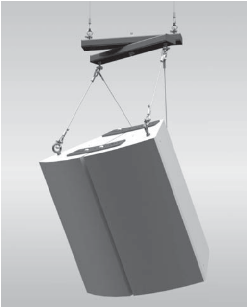
3 Point suspension using adjustable tilt Cable Kit, bridle at the rear and SAS-1WA-20 One way Array Rigging System
